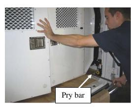
Position the entire unit according to the measurements on the following page. *Note: Maneuver the kit into position.*
